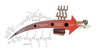
thin films with a very high degree of structural order that can be used to fabricate p-type thin film transistors with very high mobilities. We will discuss how to control charge injection in these devices through both polymer structure design, and through the intentional addition of traps that are specific for either holes or
